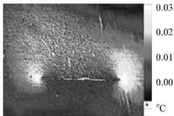
图 4.8 依赖耦合应变 - 温度场的振 - 声调制的实验结果 (来源于 Klepka A. , Staszewski WJ. , Jenal R. , Szwedo M. , Uhl T. , and Iwaniec J. 2012a. Nonlinear acoustics for fatigue crack detection experimental investigations of vibro - acoustic wave modulations. Structural Health Monitoring 25, 197 - 211, © 2012 Sage Publications) (续) b) 温度和时间
