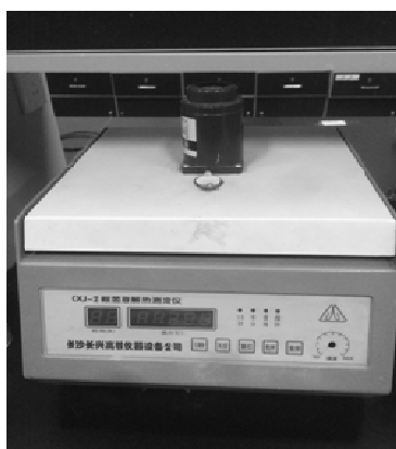
Fig. 2-2 Chemical reaction heat tester (Mode CXJ-2)
