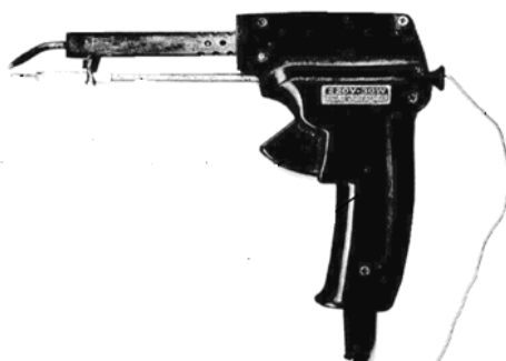
Figure 2.28 Automatic Tin Feeding Machine 自动送锡电烙铁
