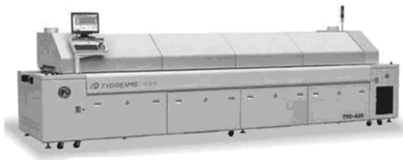
Figure 2.36 Reflow Soldering Machine 回流焊接机
