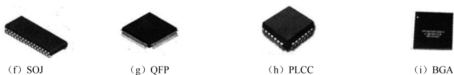
Figure 1.25 Common Various Types of Packages of ICs IC 的常用封装类型 (续)
